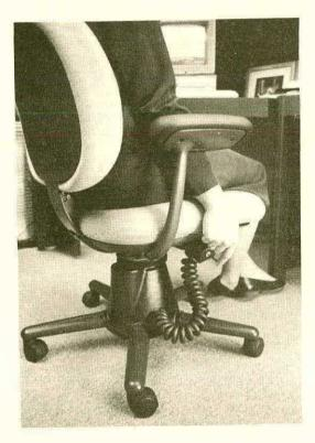
wheelchair and propels herself short distances by pushing along the edge of the work surface. After three months of use, a repair and design modification was made, however, the chair has performed reliably since then. It is believed that there is a large able-bodied market for this device since there are many who take advantage of pneumatic cylinder chairs who cannot remove their weight from the seat in order to elevate.
