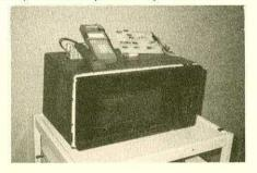
Photo 1: Working Prototype of the Intelligent Microwave Oven with hand held scanner and microcomputer.
